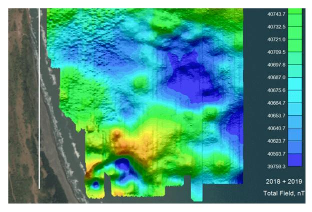
Strong volcanic underlying geology created widely varying TF signals. The Total Gradient, or Analytic Signal (AS) map was computed from the TF grid, suppressing most geological effects, and allowing many near-surface targets to be identified. A zoomed area of the above map is shown below.
