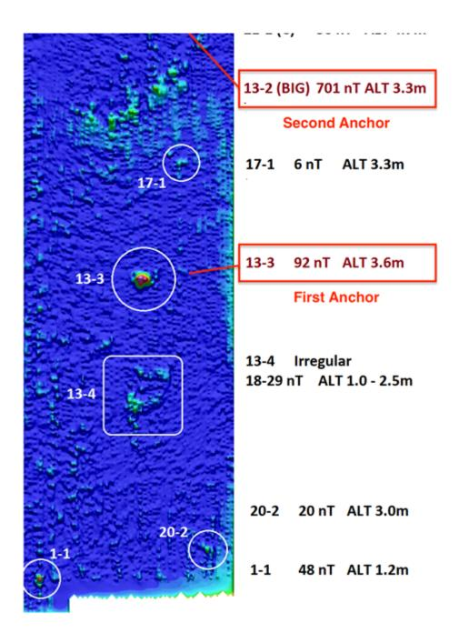
Large amounts of highly mobile sediment in the bay visually obscured all targets that were investigated. Furthermore, the sediment (sand and clay mix) was strongly magnetic due to magnetite content, and prevented the operation of pulse-induction metal detectors.
