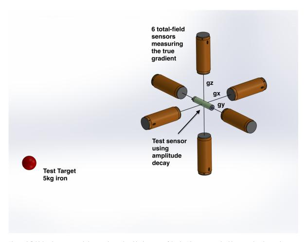
The total-field Overhauser sensor being tested was placed in the centre of the rig. Then, a magnetic object was placed several meters away, initially out of detection range. The rig was kept stationary while the magnetic object was brought closer. At each position, the value of the measured six-sensor gradient vector was recorded, along with the value of  $\tau$ , measured by the seventh sensor.
