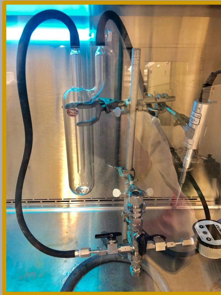
Figure 1: ExCALiBR prototype: our novel, non-aqueous lipid extractor for life detection missions
