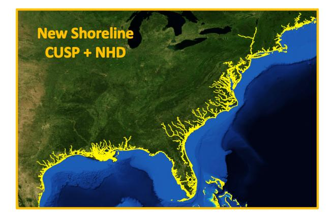
Aforementioned new shoreline has sufficient resolution to represent channels on the order of a couple of meters (see Fig.6) and incorporates the delineation of river boundaries in all the nearshore region over 20 masl.
