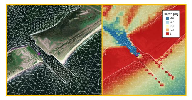
We collected  $\sim 1.5$  Tb of different bathymetry datasets (see Fig. 10). We use layers of interpolation, prioritizing the newest and highest-resolution sets in areas with overlapping of information.
