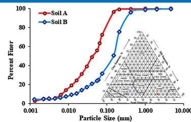
Fig.2: Grain size distribution of soil samples collected.
