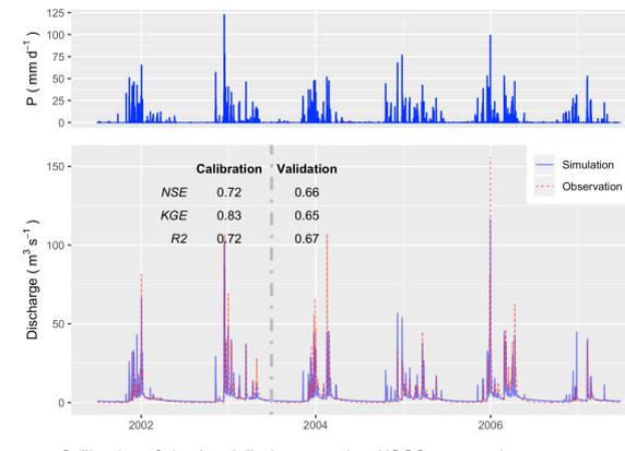
Calibration of simulated discharge against USGS gage station.
