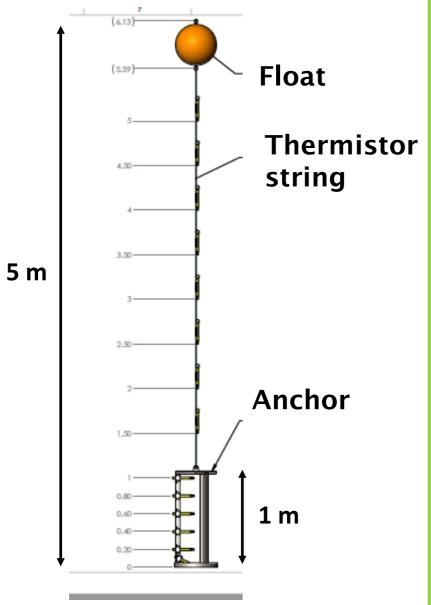
Near-bottom temperature within ASHES was surveyed using a 5-m thermistor array hanging beneath an ROV in Jun 2018. INF: Inferno vent MUS: Mushroom vent
