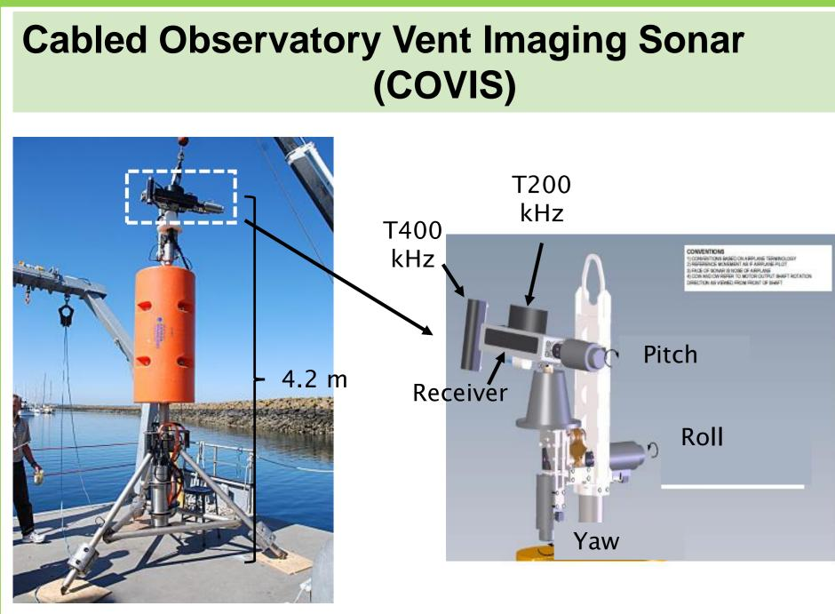
Dual frequencies: 200 kHz and 400 kHz. Sonar orientation adjustable in three dimensions
