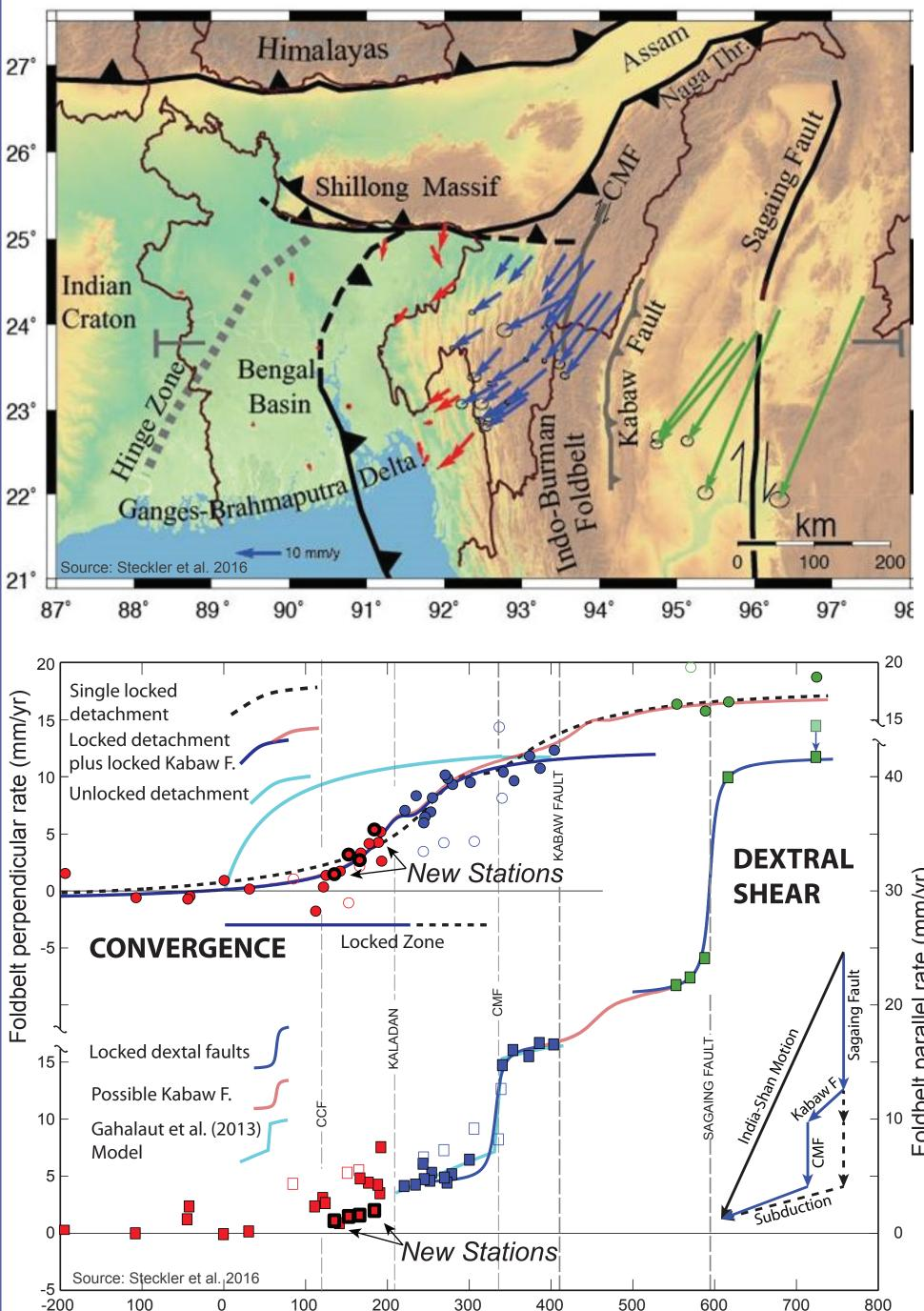
Bottom figure represents GPS velocity shortening across (circle) and shear parallel (square) to the fold belt. The velocity triangle shows the partitioning of the oblique motion between fold belt parallel and fold belt perpendicular.
