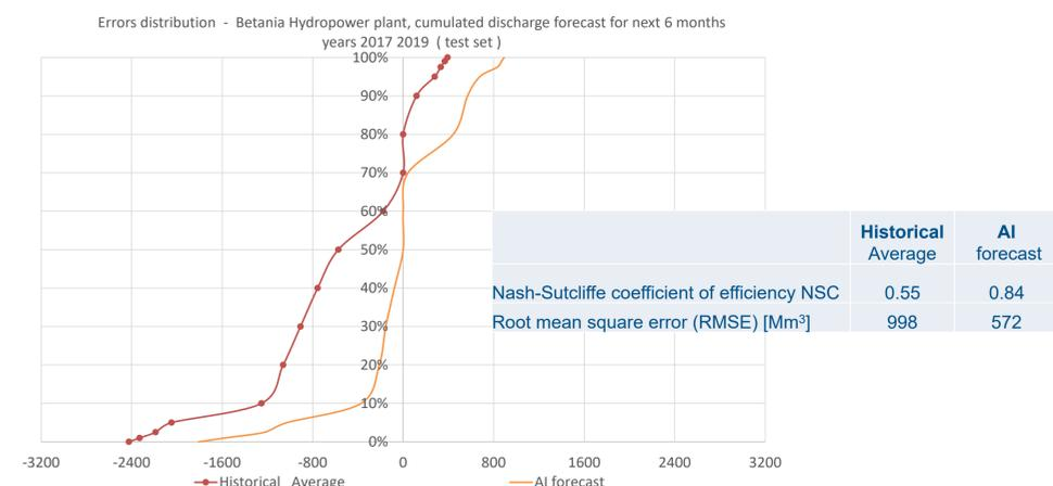
Fig 2 – Error distribution [Mm<sup>3</sup>] for 6-month forecast- Betania HPP
