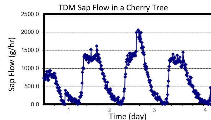
TDM probe calculated results. Graph shows three and a half days worth of data taken from a Cherry Tree taken during mid August.
