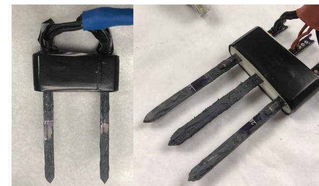
All probes are identical, having slots for both a heaters and temperature sensors. A 3D printed housing secures the probes in place. By using a 3D printed housing and multipurpose probes infinite sensor geometries can be built using the same parts; including HRM (Step D, right), TDM (Step D, left) sap flow sensors.
