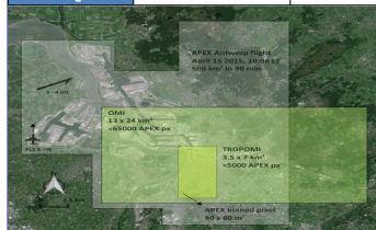
Figure 1: This figure demonstrates the satellite footprint size comparison between Aura/OMI and S5P/TROPOMI. The Airborne Prism Experiment (APEX) was an airborne flight campaign held in Antwerp, Brussels, and Liege in Belgium. TROPOMI's wide spectral coverage and the 3.5km by 7km spatial resolution bring space-based atmospheric chemistry remote sensing capability to a new, improved level (Frederick Tack et. al.).
