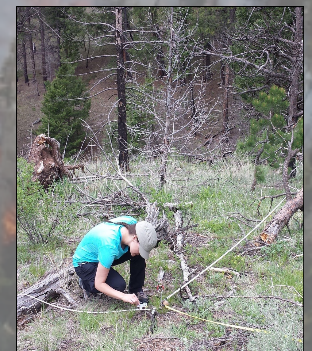
Fig. 8 Using Brown's planar intercept method to assess fuel loads.
