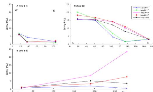
**Fig. 4. Salinity recorded in the monitoring wells adjacent to the ERT profiles. A) Profile B1; B. Profile B2; C) Profile B3. Horizontal locations are relative to the start of each ERT profile (Figures 2).**
