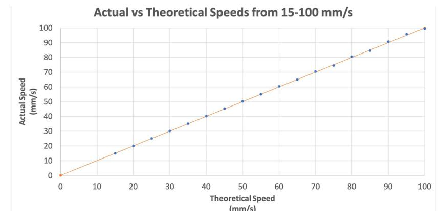
Figure 6. This is the data of the performance of the HyperRail for speeds 15-100 mm/s.
