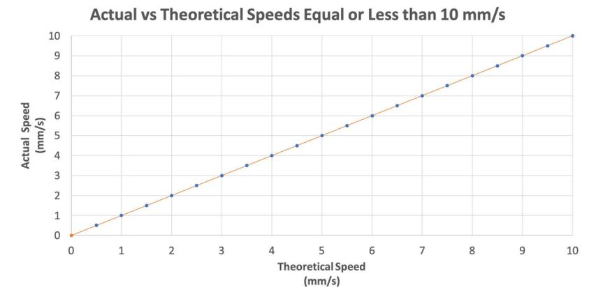
Figure 5. Data of the performance of the HyperRail for speeds less than or equal to 10 mm/s.
