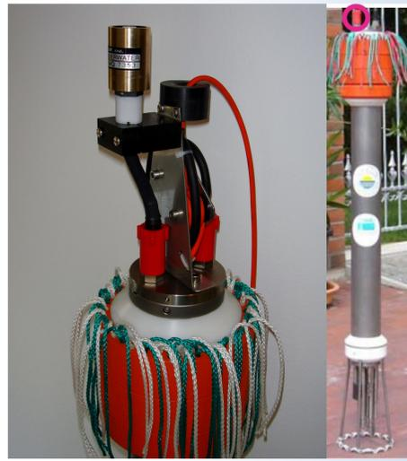
PAR sensor (LI-COR LI 192 SA) is also installed on top of a micro-structure probe (MSS90 Sea&Sun). The probe records data from each sensor with a frequency 1024 Hz. At the beginning of vertical cast, the probe records PAR in air for at least 10 s. Vertical distance between PAR sensor and the pressure sensor is 1.2 m, accounted for in data pairs (depth, PAR).
