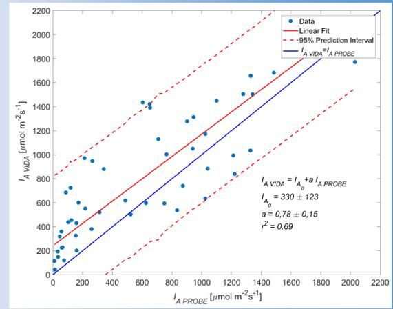
PAR data measured on VidA (15 min  $\langle \rangle$ ) versus PAR data retrieved by casts by MSS90 probe (10s  $\langle \rangle$ ) from July 2011 to December 2015. The majority of PAR values on VidA were higher than probe values. PAR sensor on the buoy is at height 4.5 m above the sea surface, while PAR sensor on the probe is 1 m above the sea surface at most, influenced by the shadow of the research boat (12 m in length).
