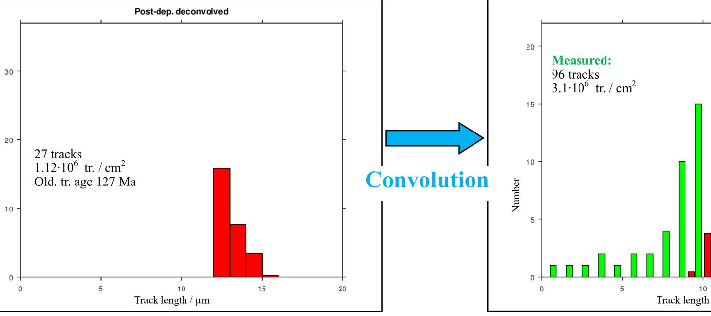
Track length / µm The convolved postdepositional histogram shown with the measured histogram. Convolution broadens the deconvolved histogram.
