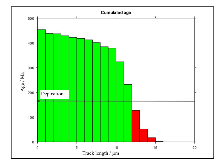
Cumulation of track ages of the deconvolved histogram from long to short tracks. Ages are calculated using a diagram [5] relating mean track length to surface track density. Tracks younger than the deposition age are identified.
