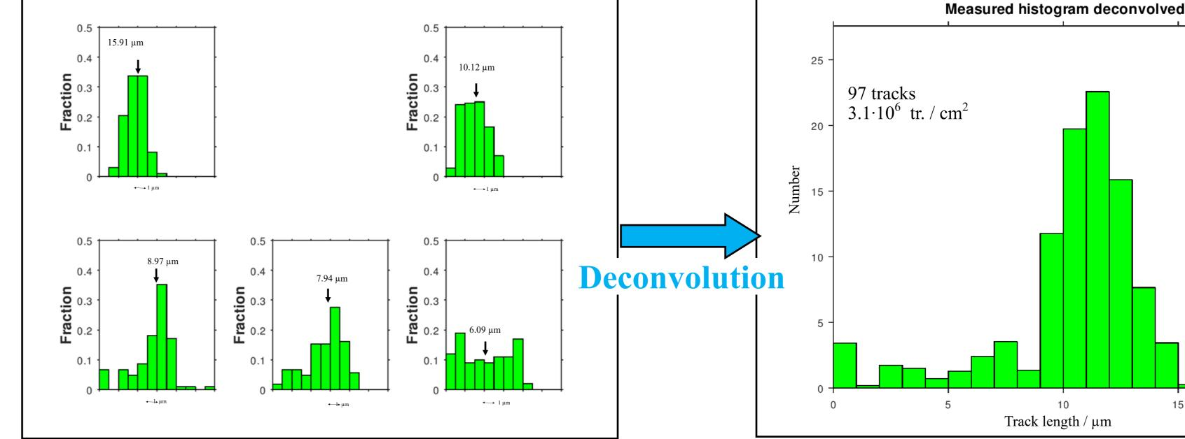
A filter is placed with its center on each bin of the measured histogram. The filters are scaled so their sum matches the measured histogram. The tracks in the histogram of scaling factors are organized chronologically, short tracks being older than long tracks. Shortening increases by anneal-
