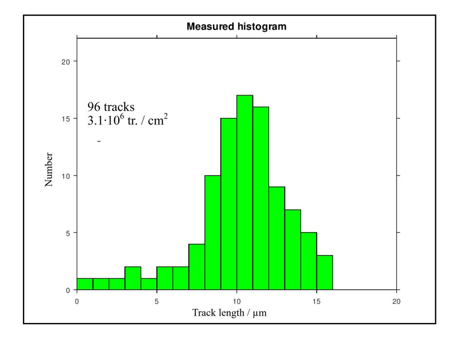
The measured fission track length histogram is considered as composed of induced track length distributions [2] after laboratory annealing [3] and [4],
