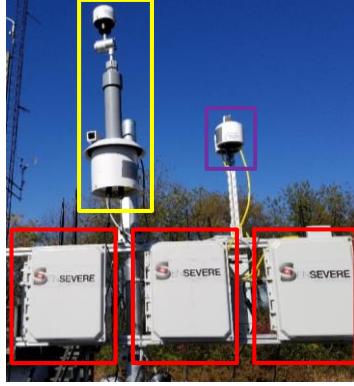
Figure S.1: Several RAMP monitors (red boxes) with connected Met-One NPM (yellow box) and PurpleAir (purple box) PM 2.5 sensors.
